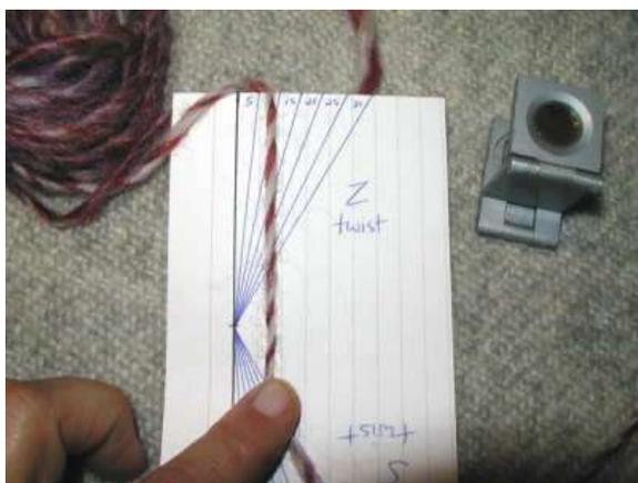
This picture illustrates measuring the twist angle of a singles yarn. I've anchored the yarn in a small slit at the top of the card, and I hold it straight, parallel to the lines on the card, with my finger. Don't pull it tight—just hold it under enough tension to keep the yarn reasonably straight. More tension than that will stretch the yarn, making the angles measure more shallow than they really are.
